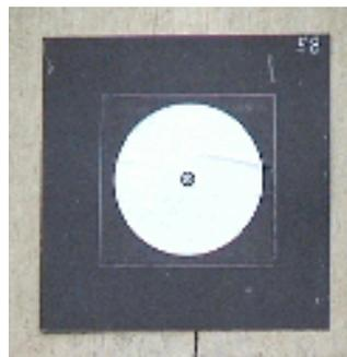
Fig. 2: Signalized points: close-up and part of measurement image
