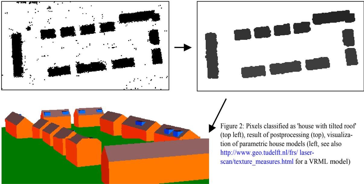
Figure 2: Pixels classified as 'house with tilted roof' (top left), result of postprocessing (top), visualization of parametric house models (left, see also [http://www.geo.tudelft.nl/frs/laser-scan/texture\\_measures.html](http://www.geo.tudelft.nl/frs/laser-scan/texture_measures.html) for a VRML model)
