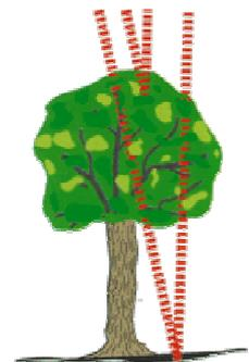
Figure 1: First- and last-pulse from a tree
