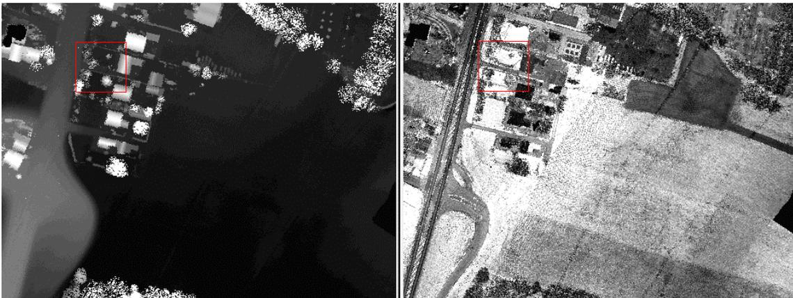
Figure 2. Laserscanner data: height and reflectance image.
