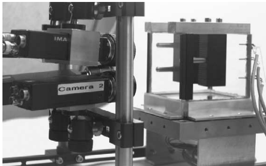
Fig. 4. Four-camera 3-D PTV arrangement, fluid cell with calibration body.
