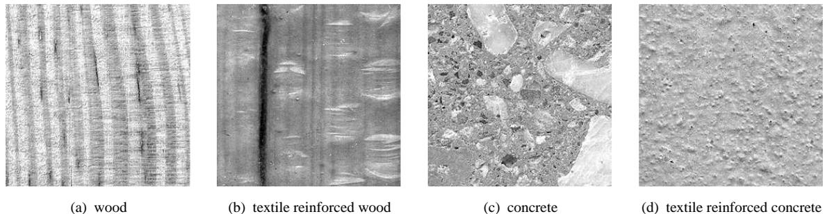
Figure 2: Textures of natural surfaces on test objects in civil engineering material testing.
