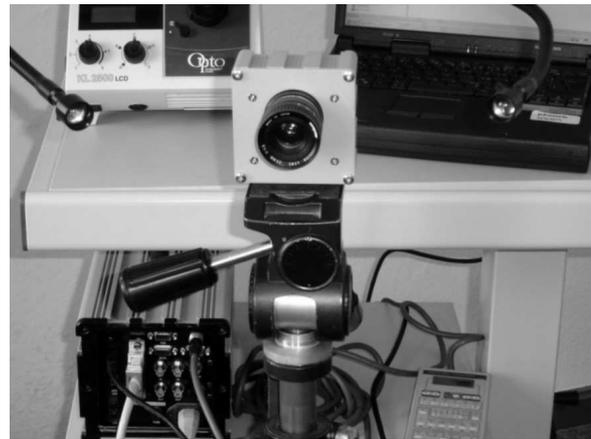
(b) Fast Cam Ultima (High Speed Camera)
