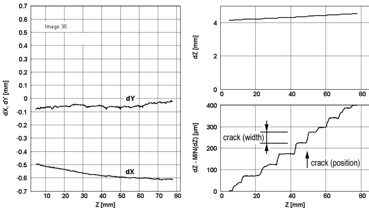
Figure 5: Results of 3-D deformation analysis.
