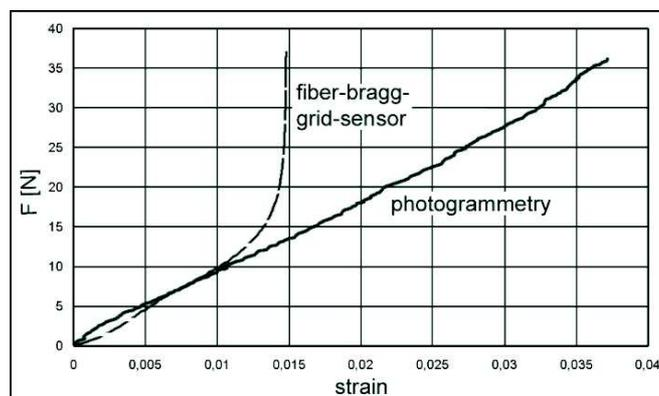
Figure 7: Verification of values of a fiber-bragg-grid-sensor and photogrammetry.
