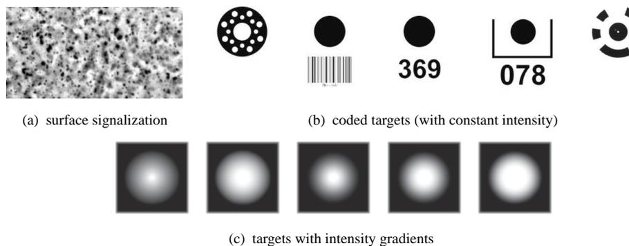
Figure 3: Artificial signalization of discrete points and surfaces.
