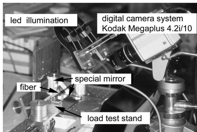
Figure 6: Test stand for calibration of fiber-bragg-grid-sensors with digital photogrammetry (mirror photogrammetry).
