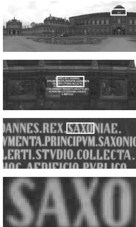
Fig. 4: Resolution potential of the camera EYESCAN M3 illustrated through 4 zoom steps
