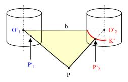
Fig. 10: Epipolar line geometry of panoramas
