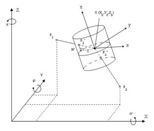
Fig. 5: Geometrical model (Definition of used variables in Schneider & Maas 2003b)
