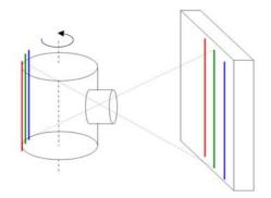
Fig. 3: Principle of digital panoramic image accuisition
