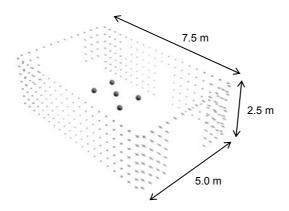
Fig. 9: Object points of calibration room of AICON 3D Systems GmbH incl. camera positions
