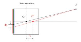
Fig. 6: Model deviations (e<sub>1</sub>: eccentricity of projection centre)
