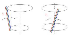
Fig. 7: Model deviations  $(\gamma_1, \gamma_2: \text{Non-parallelism of CCD line, 2 components})$
