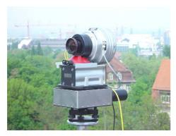
Fig. 4: Digital panoramic camera EYESCAN M3
