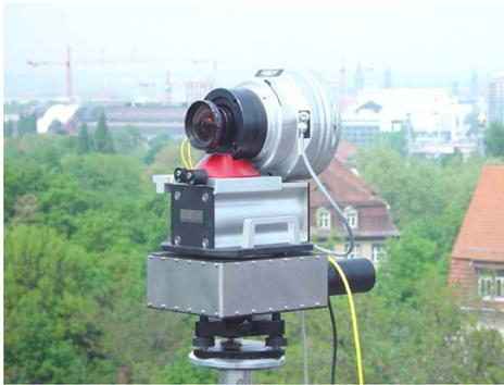
Fig. 4: Digital panoramic camera EYESCAN M3
