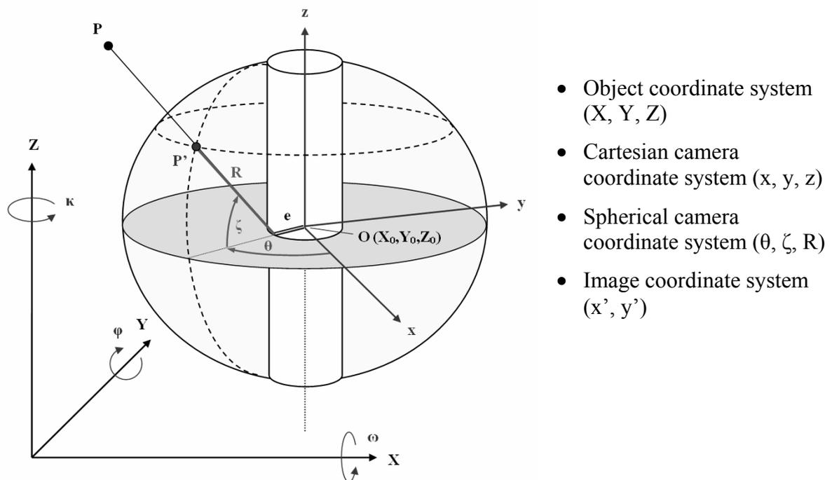
Figure 3: Geometrical model based on spherical coordinates
