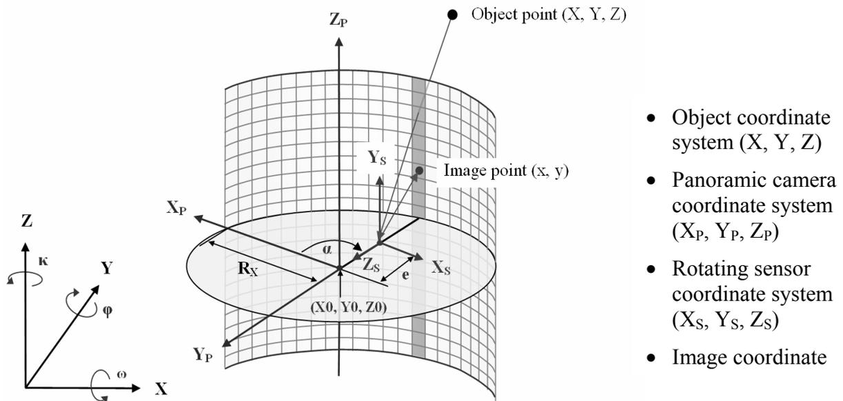
Figure 5: Full-spherical projection principle based on a rotated sensor coordinate system
