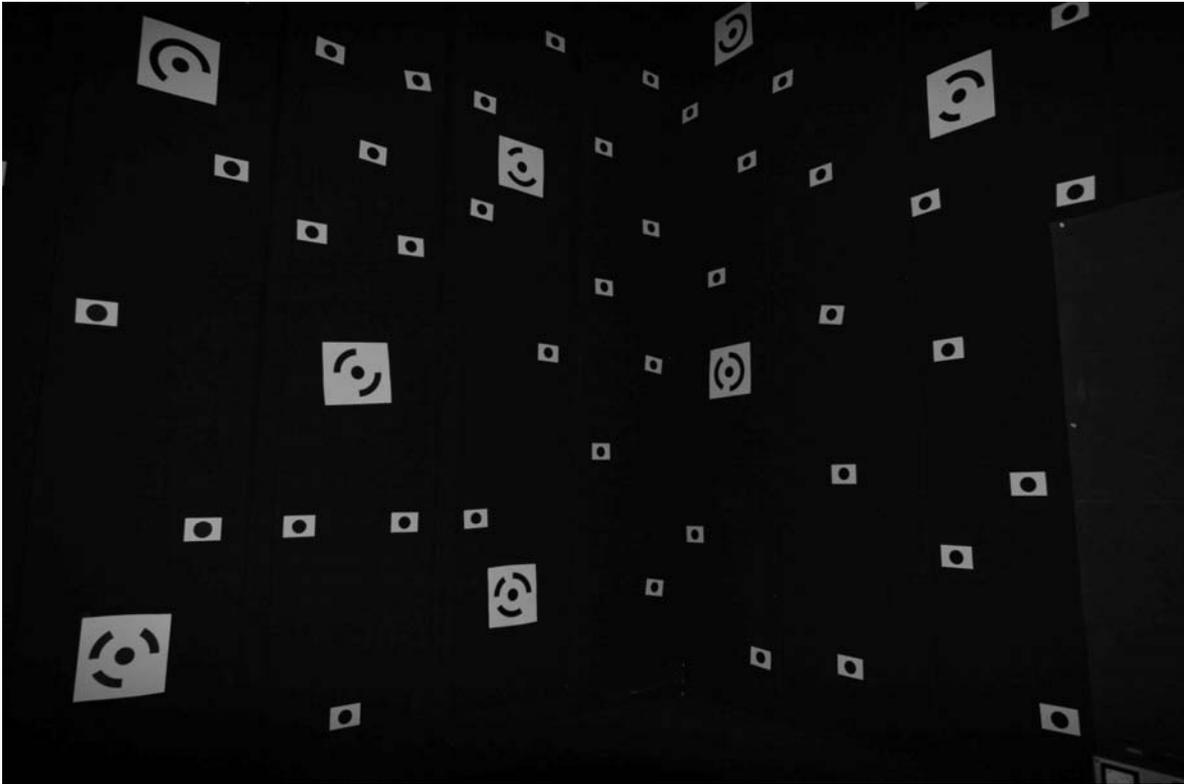
Fig. 3.2 – View inside the test facility with calibration targets on the walls.
