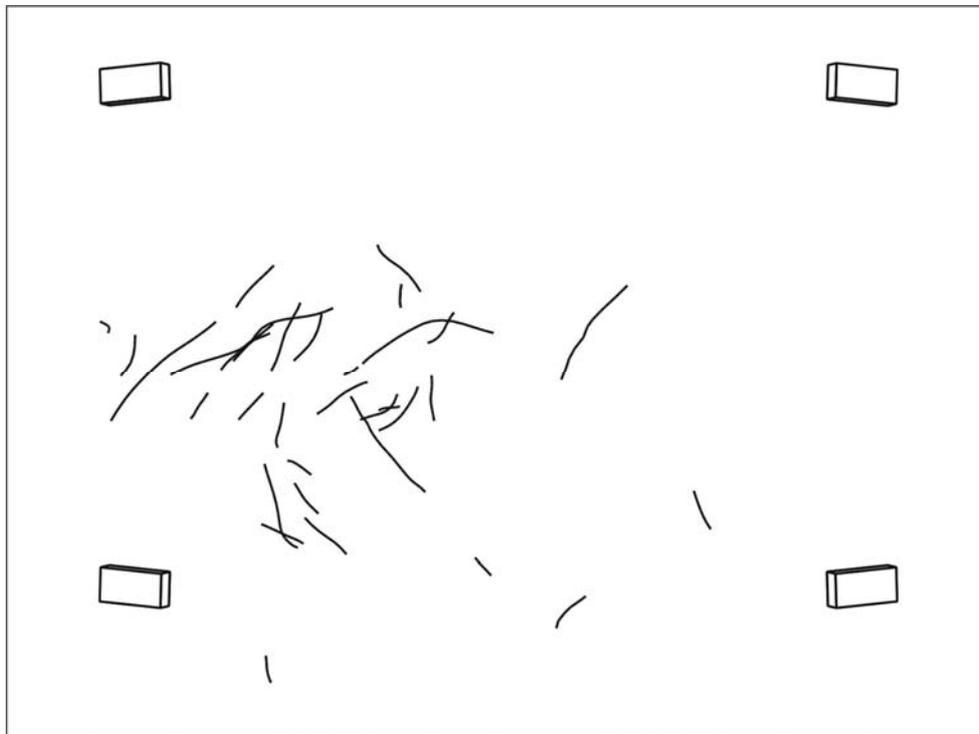
Fig. 4.2 – Example of the reconstruction of selected particle tracks inside the test cell in a forced convection flow. The boxes in the corners show the positions of the cameras.
