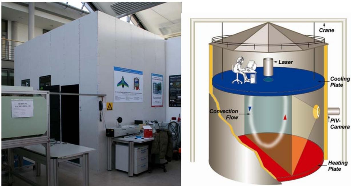
Fig. 3.1 – The experimental test facility with 4.2 m length, 3.0 m width and 3.6 m height seen from outside (left) and the schematic sketch of the BOF (right).
