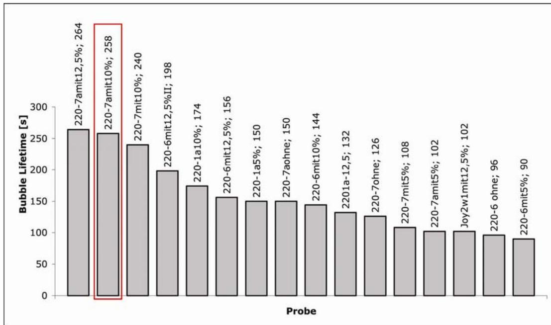
Fig. 3.3 – Lifetime measurements of helium filled soap bubbles in a test chamber. The lifetime was determined by counting the absolute number of bubble tracks in a certain time interval by means of CCD-camera images. The red framed probe with a life time of 258 s is used because of its maximum bubble generation rate.
