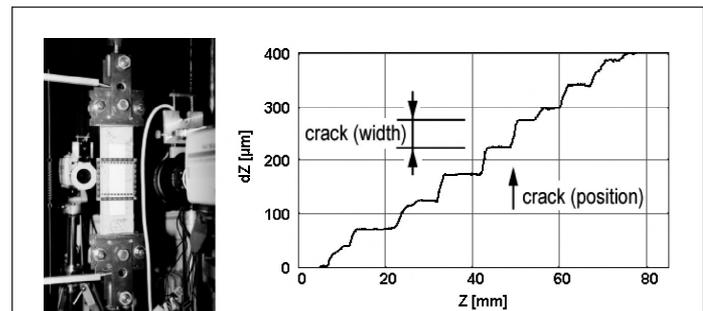
Figure 4. Imaging configuration for double-sided crack detection, probe profile obtained by deformation vector field analysis (approximately 1,600 points).
