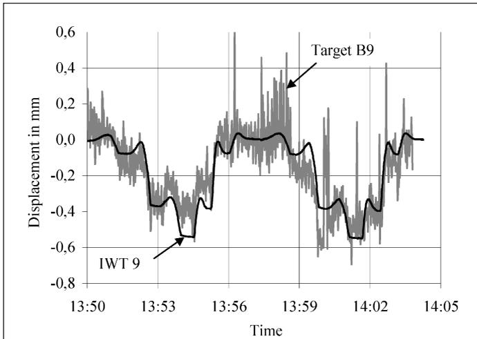
Figure 8. Comparison of inductive gauge (IWT 9) and photogrammetric (B9) deformation measurements at one target on the bridge shown in Figure 6 over a 15 minute load test with two load cycles (Albert *et al.*, 2002).
