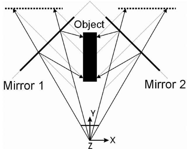
Figure 2. Photogrammetric recording scheme with mirrors.
