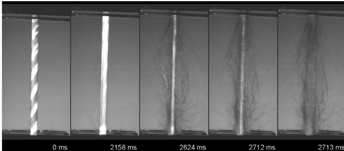
Figure 10. Five out of 4,000 images of a 1,000 Hz highspeed camera image sequence showing the failure of a glass fibre roving for textile reinforcement of concrete parts.
