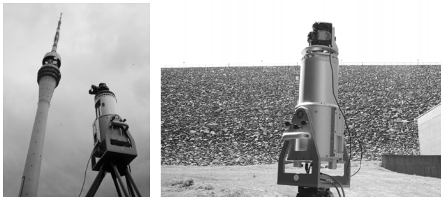
Figure 1: Laserscanner Riegl LMS-Z420i for deformation analysis of towers and water dams
