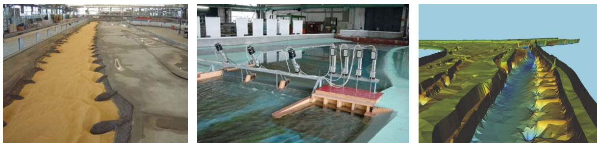
Figure 1 : Test bed of a river model, measurement devices (non contact less), generated 3D model (source BAW)
