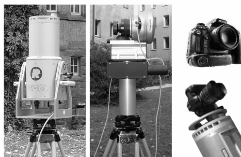
Figure 8. Combined devices (Riegl laser scanner LMS-Z420i, panoramic camera Eyescan M3, Kodak 14n, Nikon D100)
