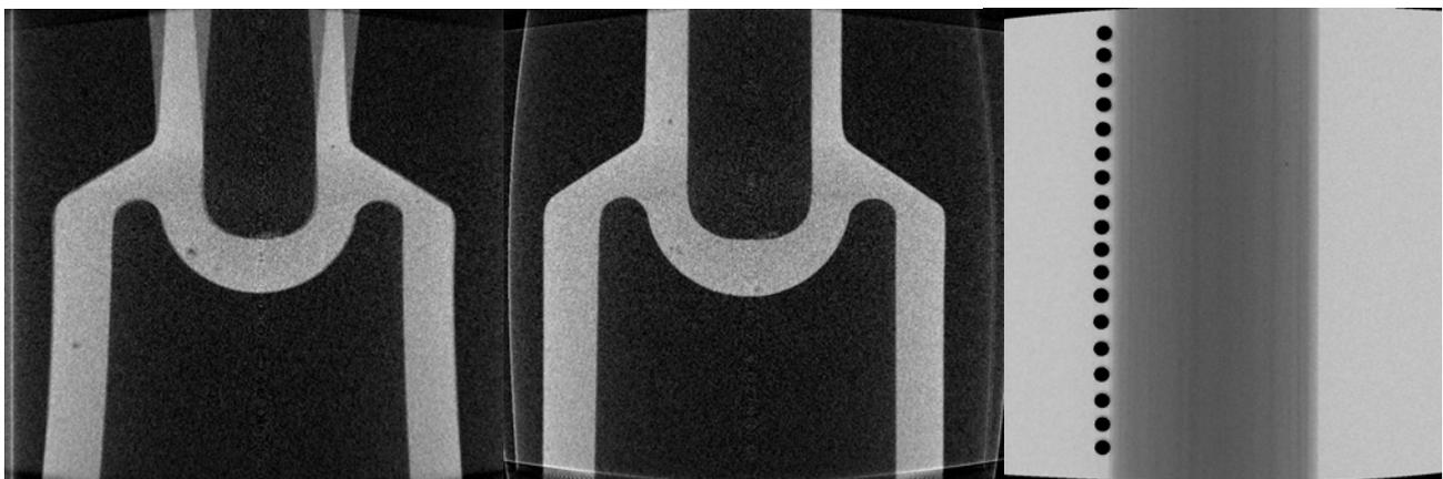
Figure 5: (a) dejusted and (b) correct sample slice along the rotation axis, (c) calibration object
