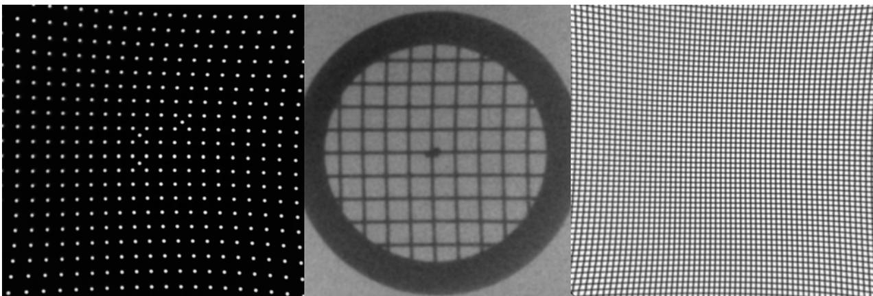
Figure 3: Calibration objects a: grit (3x3 mm), b: board (300x300 mm) and c: grit (10x10 mm)
