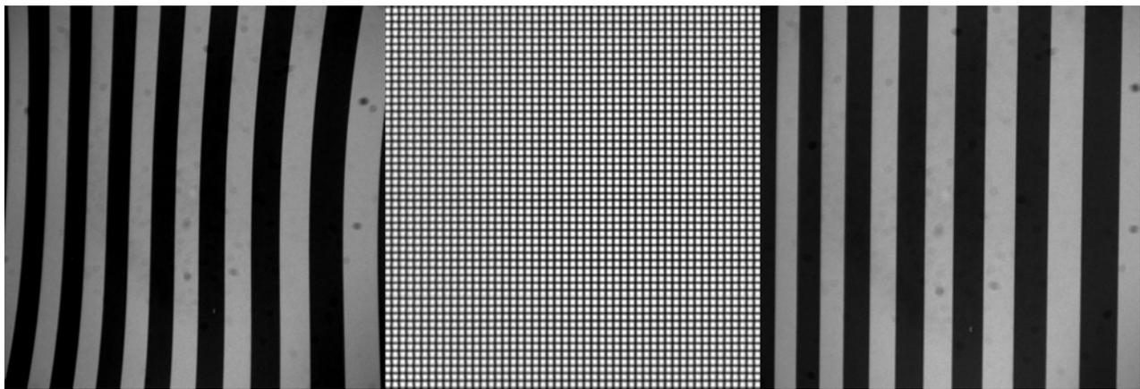
Figure 4: Verification with a calibrated line sample a: distorted image, b: rectify reference and c: rectify image
