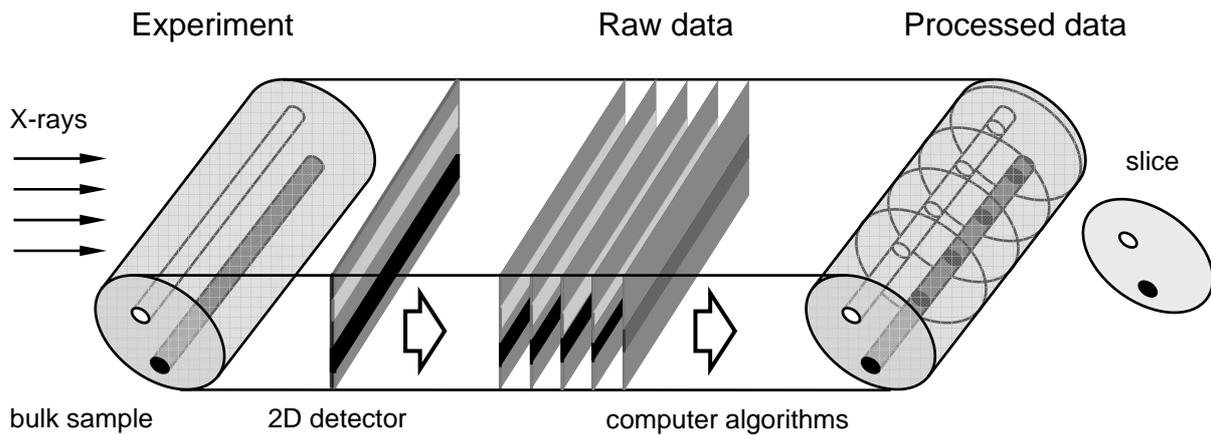
Figure 2: Principle of computer tomography
