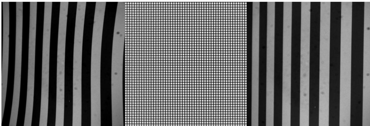
Figure 4: Verification with a calibrated line sample a: distorted image, b: rectify reference and c: rectify image
