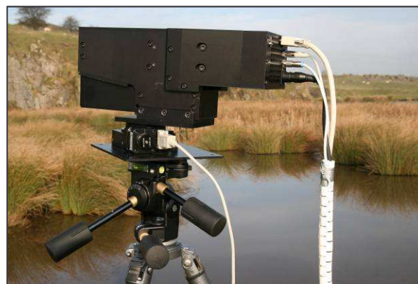
Figure 1. HySpex SWIR-320m hyperspectral imager.
