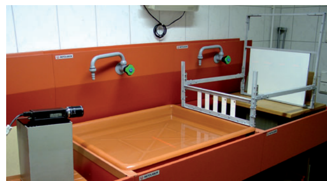
Figure 7: A test setup for the wave detection system with two projection planes.
