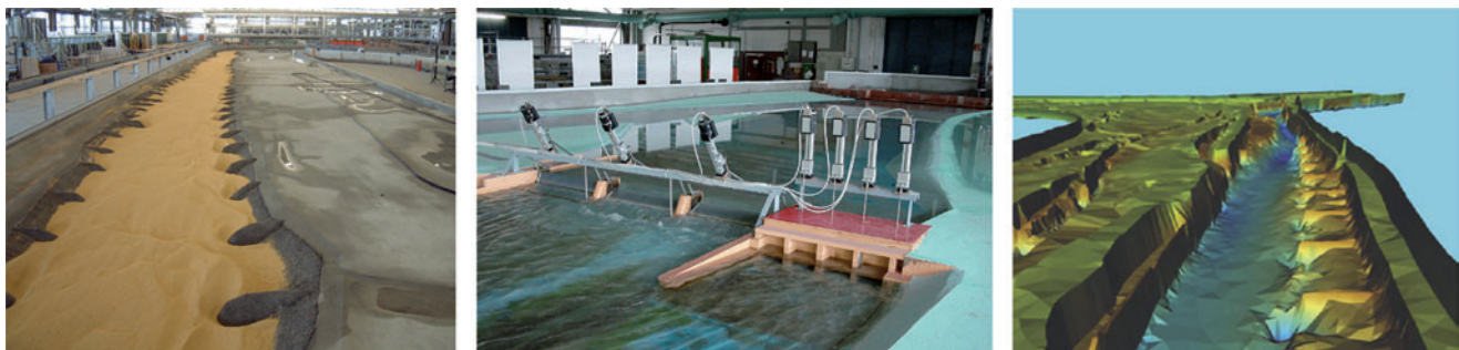
Figure 1: Test bed of a river model, pointwise gauge measurement, generated 3D model (source BAW).
