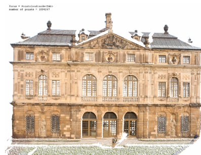
Figure 10. Point cloud of scan position 3 coloured with photo 96 oriented with SIFT keypoints
