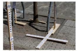
Figure 1: Detail view of markers (encoded and uncoded) placed around a tree
