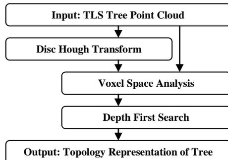
Figure 2. Processing scheme outline for topology extraction.
