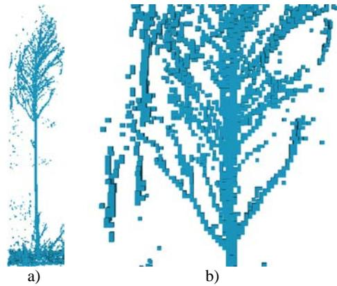
Figure 3. Voxel space representation of raw point cloud.
