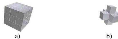
Figure 4. Voxel with a) 26-adjacency and b) 6-adjacency.
