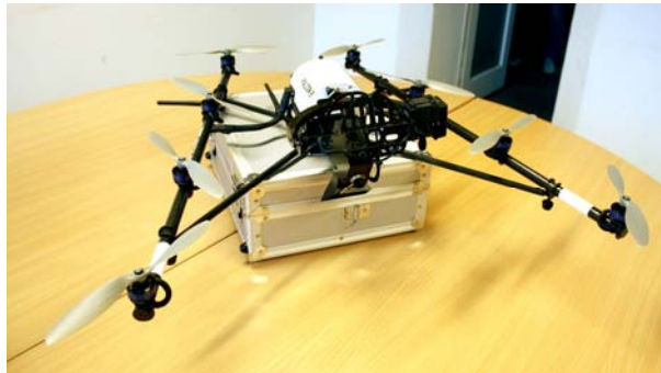
Figure 4. Unmanned aerial vehicle (UAV) Ascending Technologies Falcon 8 with mounted OPZ demonstration system
