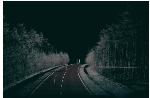
Figure 7. Scan result of a land road (206 meter)
