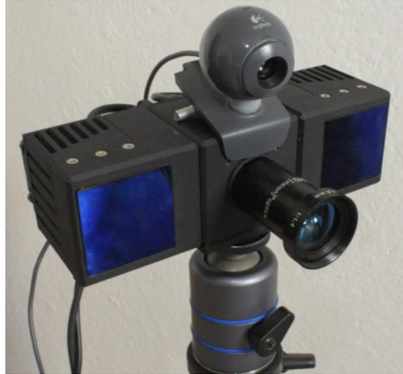
Figure 1. Sensor configuration. PMD CamCube and RGB camera Logitech C200 on top.
