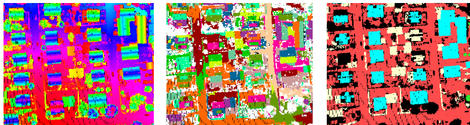
Fig. 2: Raw point clouds (left), planar segments (middle), Extracted roofs (right): cyan & white - building, green – vegetation, red – terrain, black – non segmented point patches
