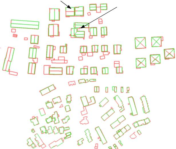
Figure 8: Visual appearance of roof models: red - 3D roof models reconstructed from high density data, green - with low density data (for the clarity, aerial view is chosen)
