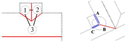
Figure 3: Convergence of Ridge-lines and Step-edges, at a closed cycle, (schematic diagram): red - ridges, blue - step-edges
