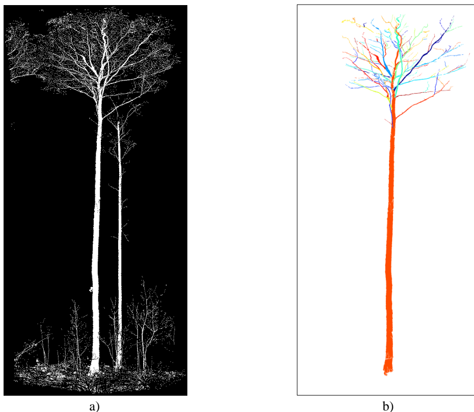
Figure 1: a) Range image cropped to bounding box. b) Manually enhanced label image, each color denotes a connected component determined by connected component labeling on the range image.
