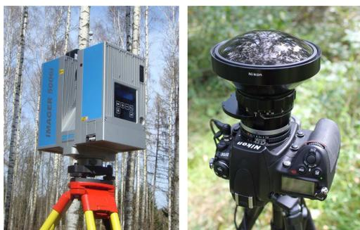
(a) Z+F laser scanner *Imager 5006i* (b) Nikon D700 with lens Nikon Fisheye 8mm
