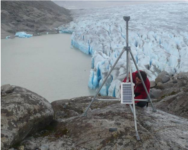
Figure 8: Time lapse camera system installation at Lago Nef Norte (Maas et al., 2012)
