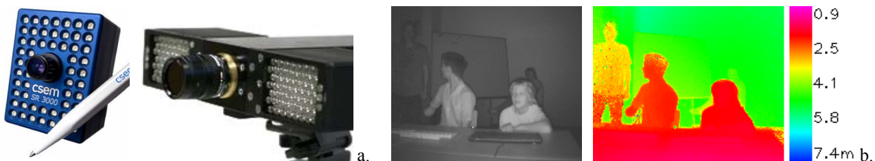
Figure 1: a. Left: SwissRanger 3000 (CSEM, 2006). Right: PMD [vision] 19k (PMD, 2007) b. Left: NIR intensity image. Right: Colour coded range image
