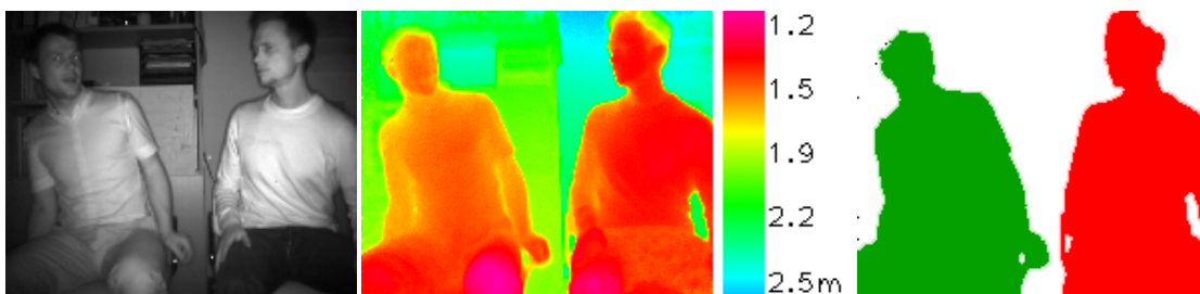
Figure 6: Left: Intensity image. Middle: Colour coded range image. Right: Image segmentation.
