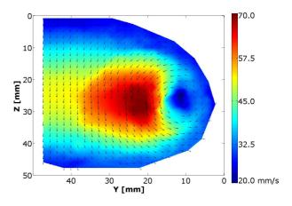
**Figure 3**: Color coded vector lengths of one half of the vortex ring (frontal view, X=const=13.14 mm).
