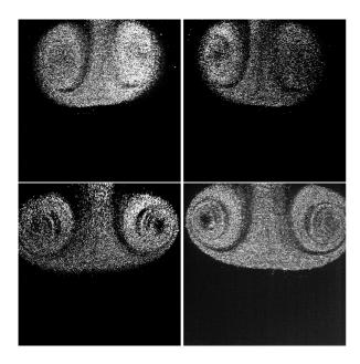
**Figure 1**: Vortex ring imaged with four high speed digital cameras equipped with telecentric lenses at one epoch.
