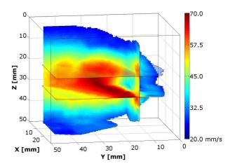
Figure 2: Cross sections of color-coded velocity in voxel space.
