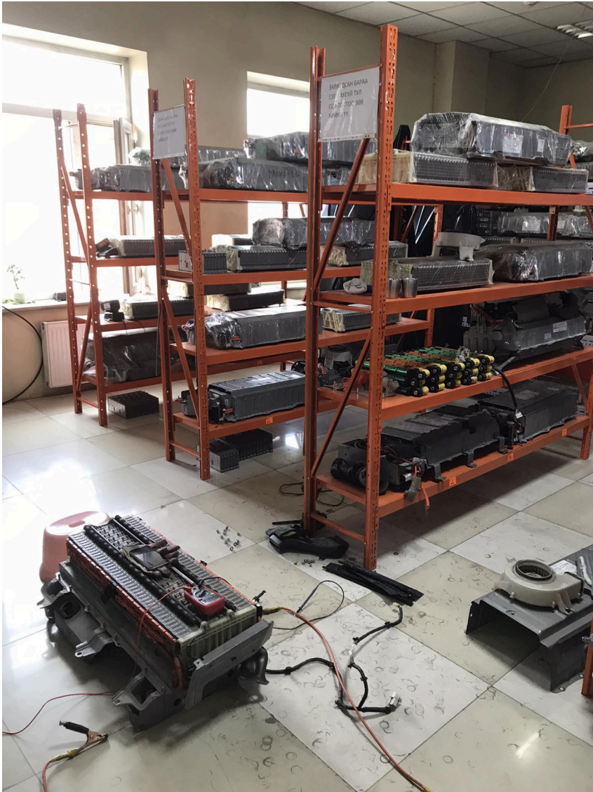
Fig. 4. Battery modules are tested, disassembled and stored in a significant number of repair shops across Ulaanbaatar. While some end-of-life modules are exported to Japan for recycling, there is no reliable information about the fate of the parts of this battery waste stream. Photo: Luisa F.S. Prates
