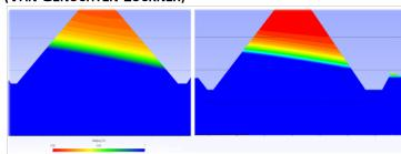
Although the water level in the dam embankment hardly changed, a significant difference from the partially saturated zone above the seepage line could be observed.
