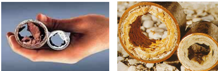
Picture 2. The impact of scale formation in pipe
