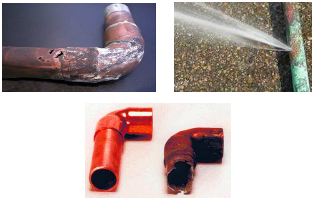
Picture 1. The impact of corrosion to the pipe
