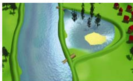
Figure 3: Scheme of a polder
