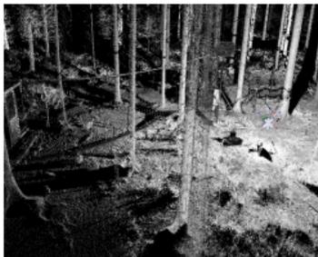
point cloud resulting from terrestrial laser scans
