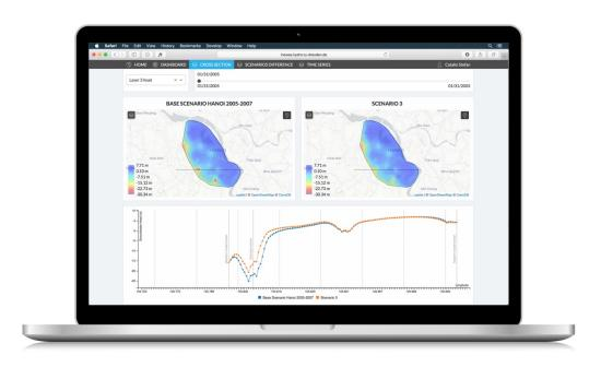
Screenshot of MODFLOW-based groundwater numerical modeling tool using the free, open source INOWAS platform
