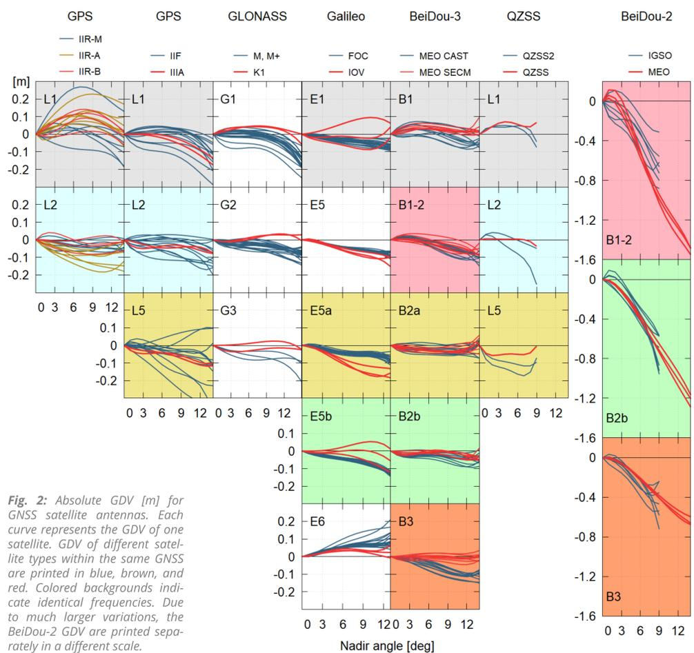
Fig. 2: Absolute GDV [m] for GNSS satellite antennas. Each curve represents the GDV of one satellite. GDV of different satellite types within the same GNSS are printed in blue, brown, and red. Colored backgrounds indicate identical frequencies. Due to much larger variations, the BeiDou-2 GDV are printed separately in a different scale.
