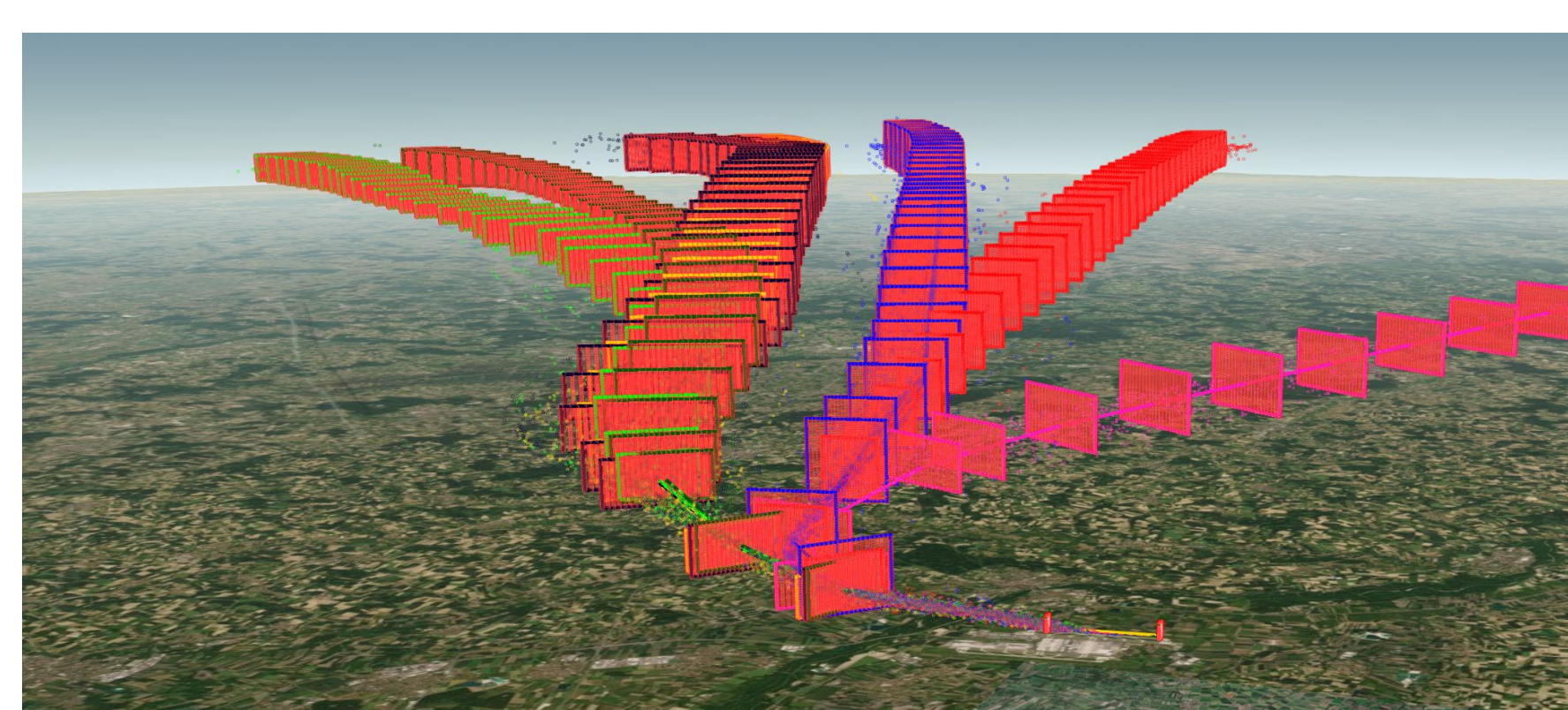
Figure 4: Departure corridors optimized based on flight performance from Munich Airport 26R [2], [3]
