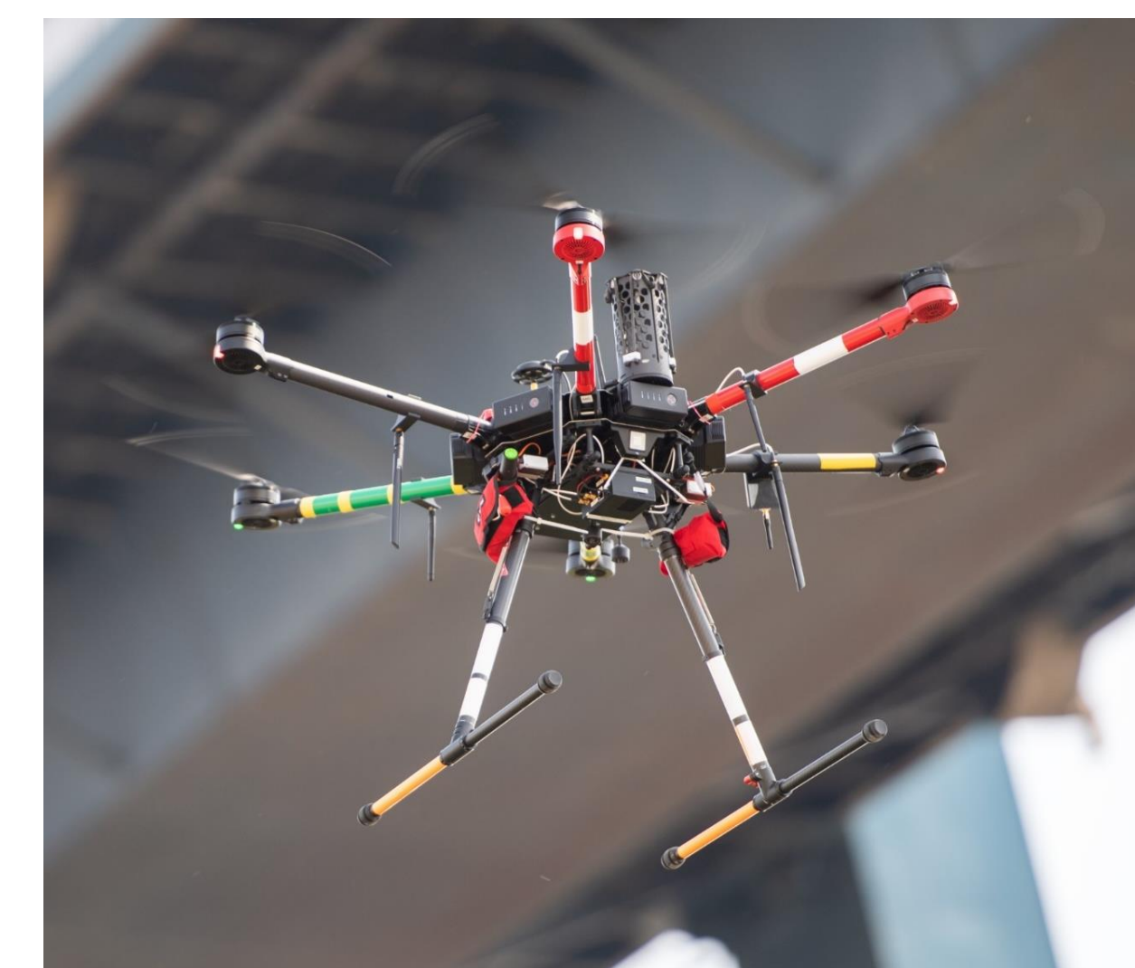
Figure 4: DLR test aircraft CDO DJI M600 (max. take-off weight: approx. 15 kg, diagonal propeller axes distance: 1,133 mm, propeller diameter 21")
