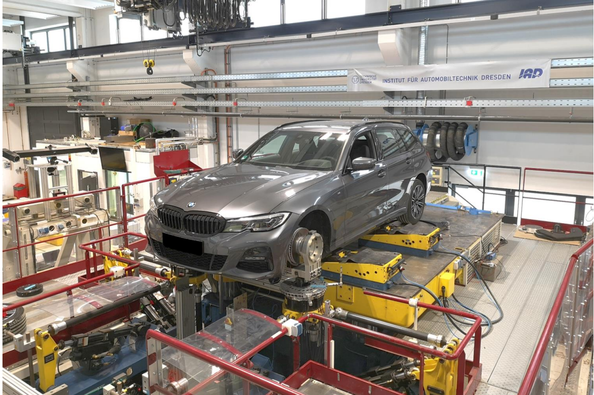
Figure 1: General view of the Suspension Motion Simulator with test vehicle
