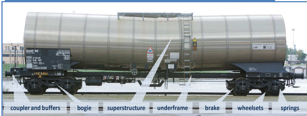
Fig. 4-1: Layout of a conventional rail freight wagon (example tank wagon)
