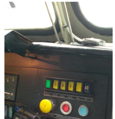
Fig. 1: ATB EG devices in the Dutch regional train Mat'64.
