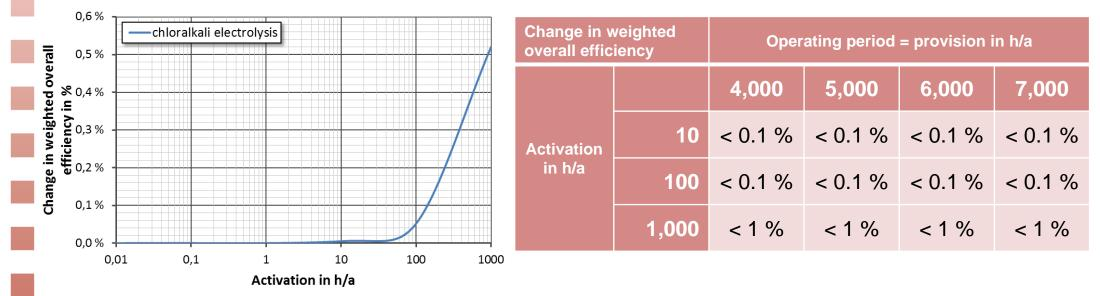
→ Activation of 1,000 h/a increases weighted overall efficiency about 0.5 %
