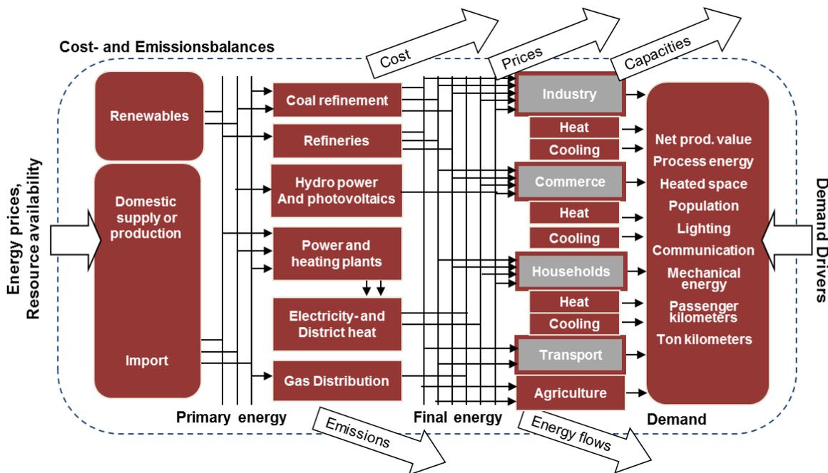
Figure 1 Simplified Reference Energy System (RES) of TIMES PanEU
