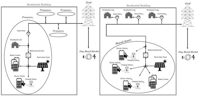
Figure 1: Individual (left) and Sharing (right) set-up of one residential building
