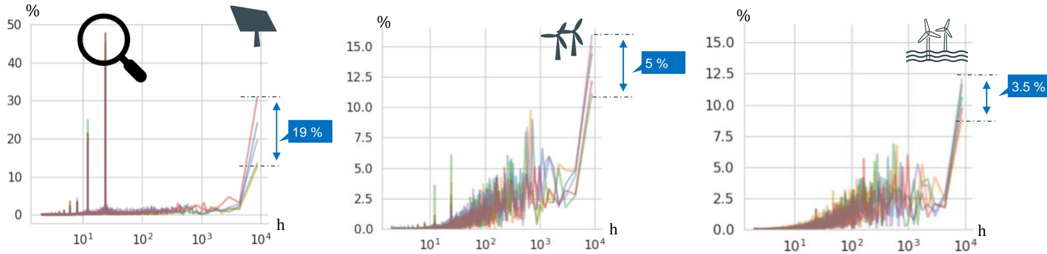
Based on the spectra, frequency cuts for the disentanglement analysis can be derived
