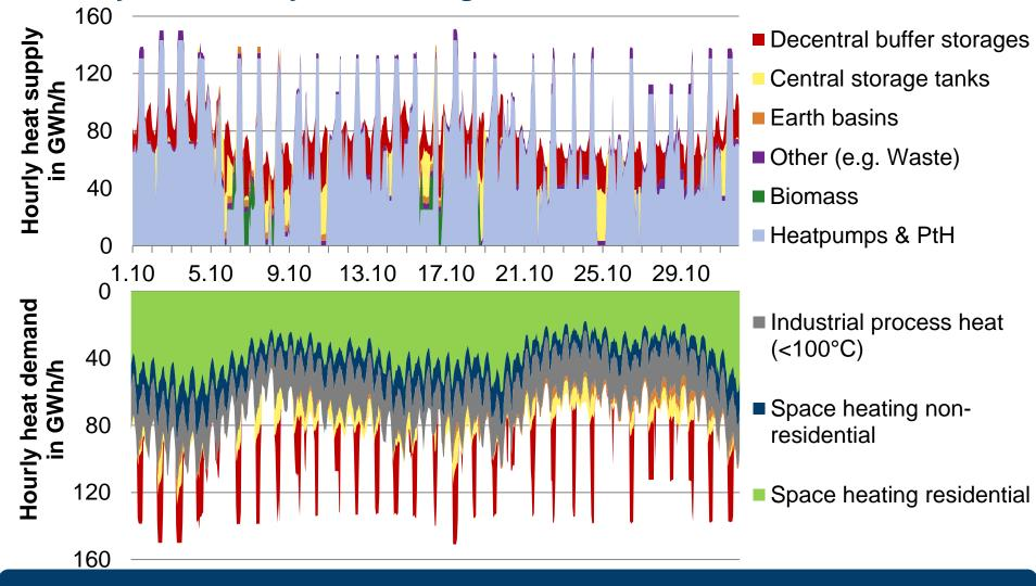
Heat storages enable flexible operation of heatpumps and PtH-applications
