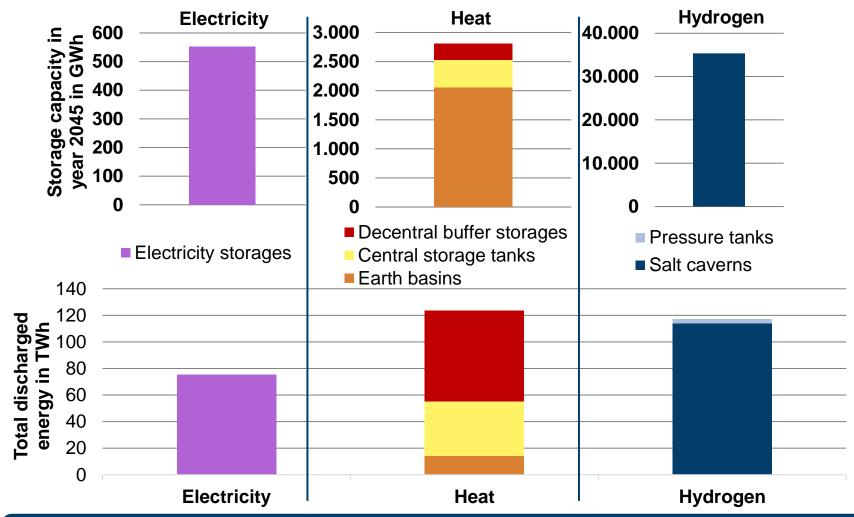
Decentral heat storages with 281 GWh capacity (10% of storage capacity), supply 68 TWh (55%) of heat
