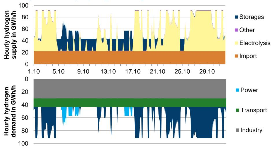
> Hydrogen storages enable flexible operation of electrolyzers
