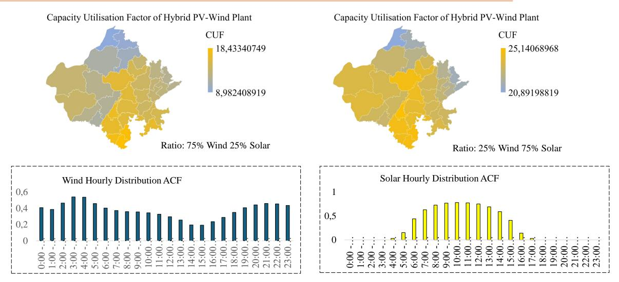
Fig. 12: Capacity Utilisation Factor of Hybrid PV-Wind Plant
